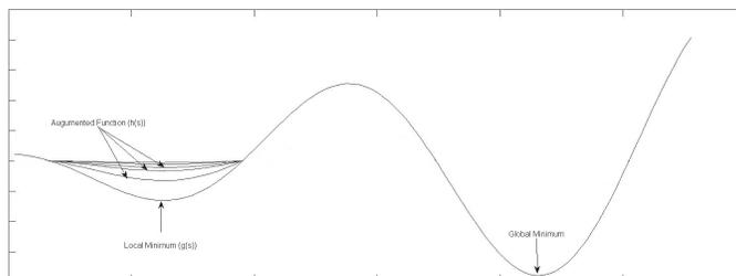
**Fig. 3.** Augmented Cost Function  $h(s)$  v.s Cost Function  $g(s)$
